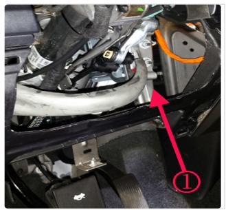
Inspect the power inverter module for possibly moving slightly against mounting bracket and creating the noise.
