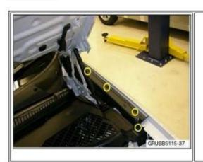
Remove the sealing trim from the left-hand side panel
