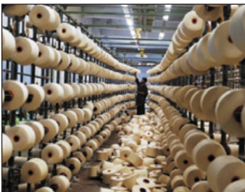
Example of Class III Location – Textile Mill
