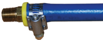
Incorrect – Push-on hose and fittings used with worm drive hose clamps
