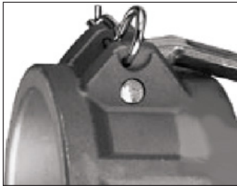
Incorrect – Wire holding locking arms in place
