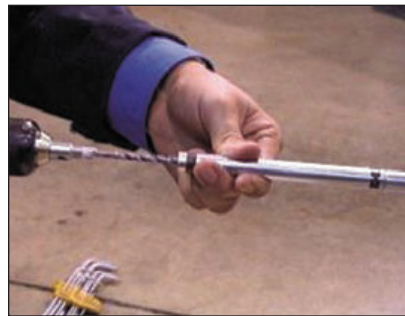
2. Install drive sleeve over the drill bit.
