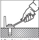
4. Place fixture in position, insert bolt and tighten.
