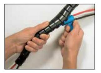
3) Slide the applicator tool through the split wire loom.
