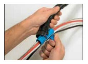
2) Place the applicator tool in one end of the split wire loom.
