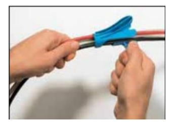
1) Insert one or more cables into the insertion slot of the applicator tool.
