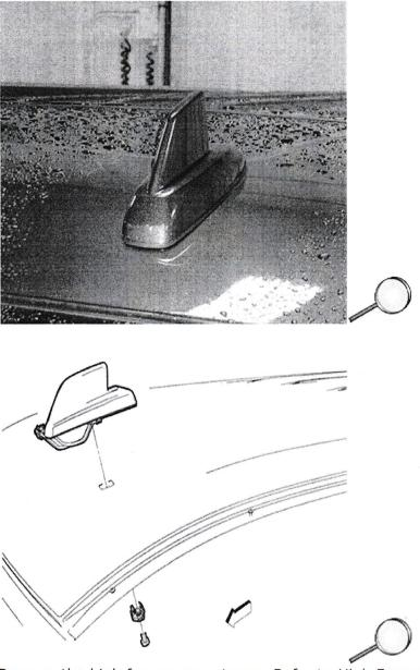
1. Remove the high frequency antenna. Refer to High Frequency Antenna Replacement in SI.
